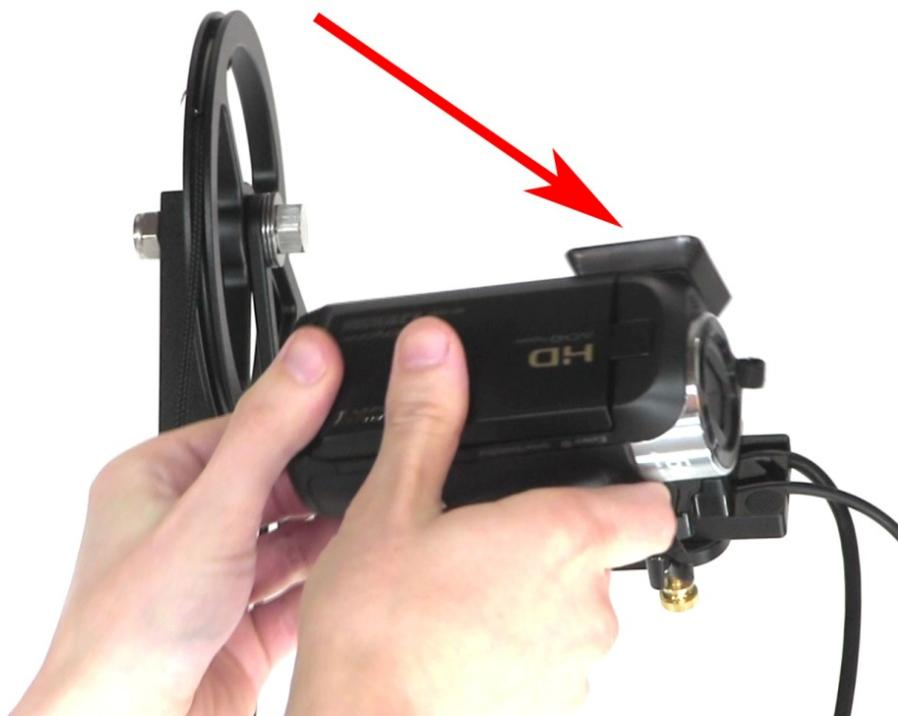
Notice how the camera already has a connection adapter attached to it. This is what you'll use to snap the camera to the quick release plate.
