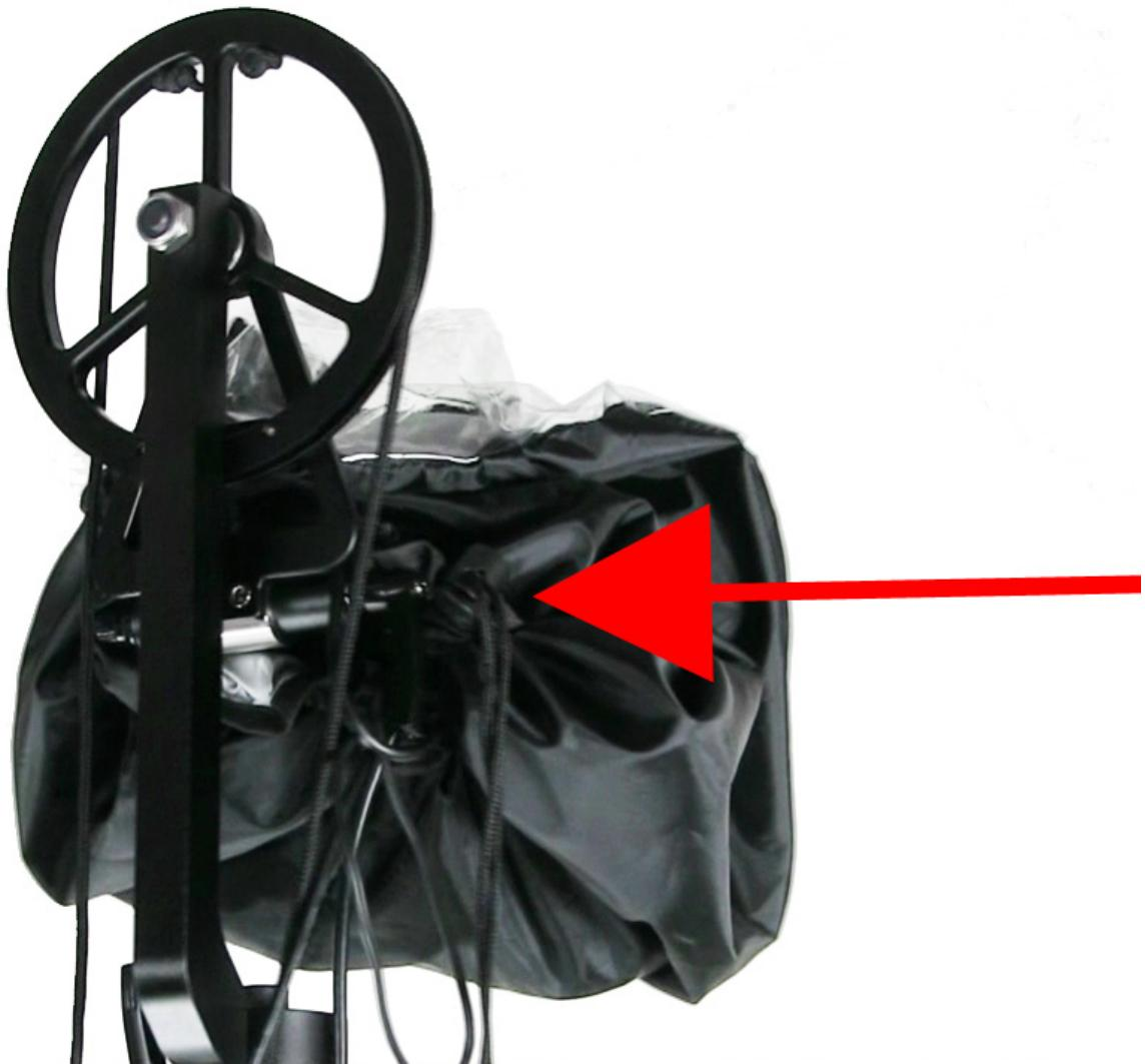
There is a cinch cord which will allow you to organize your cables, arrange the bag, and then completely close so no water can get inside. There are different ways to accomplish this, but the key is to pull the cord completely shut when finished.
