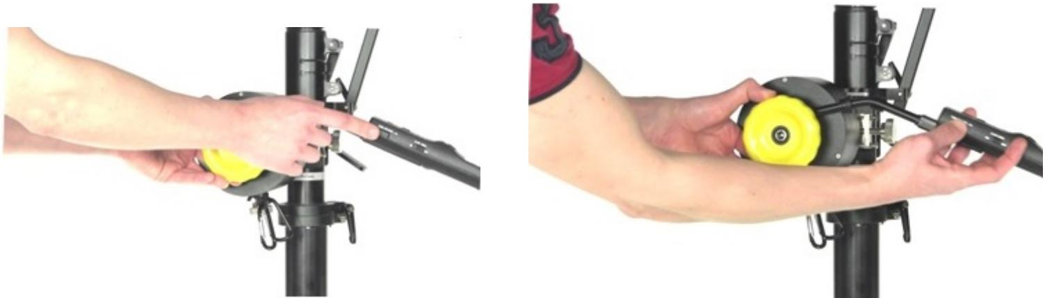
If you ever want/need to change the physical position of the remote, as it attached to the handle, you'll need to find an allen key (metric), open the screws, adjust the angle to your preference, and tighten again.
