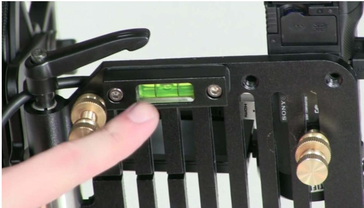
On the Hi-Pod head, from the bottom looking up, you'll find a green leveling bubble. This helps to confirm whether your shot is level with the ground before elevating.
