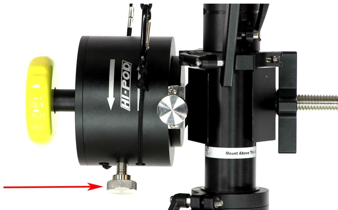
This is the screw found between the two black ropes coming out of the handle. If you lock this screw, the ropes will not pull out of the handle, nor will they retract. They will be fixed at whatever length you set them at. This is important at two points during setup.
