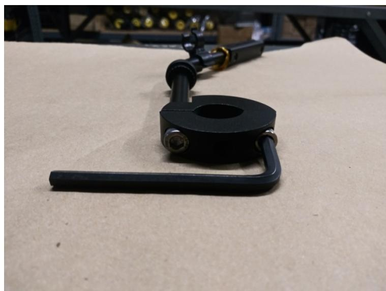
Once removed, place the split lock on the tubing between the yellow handle and the spool.
