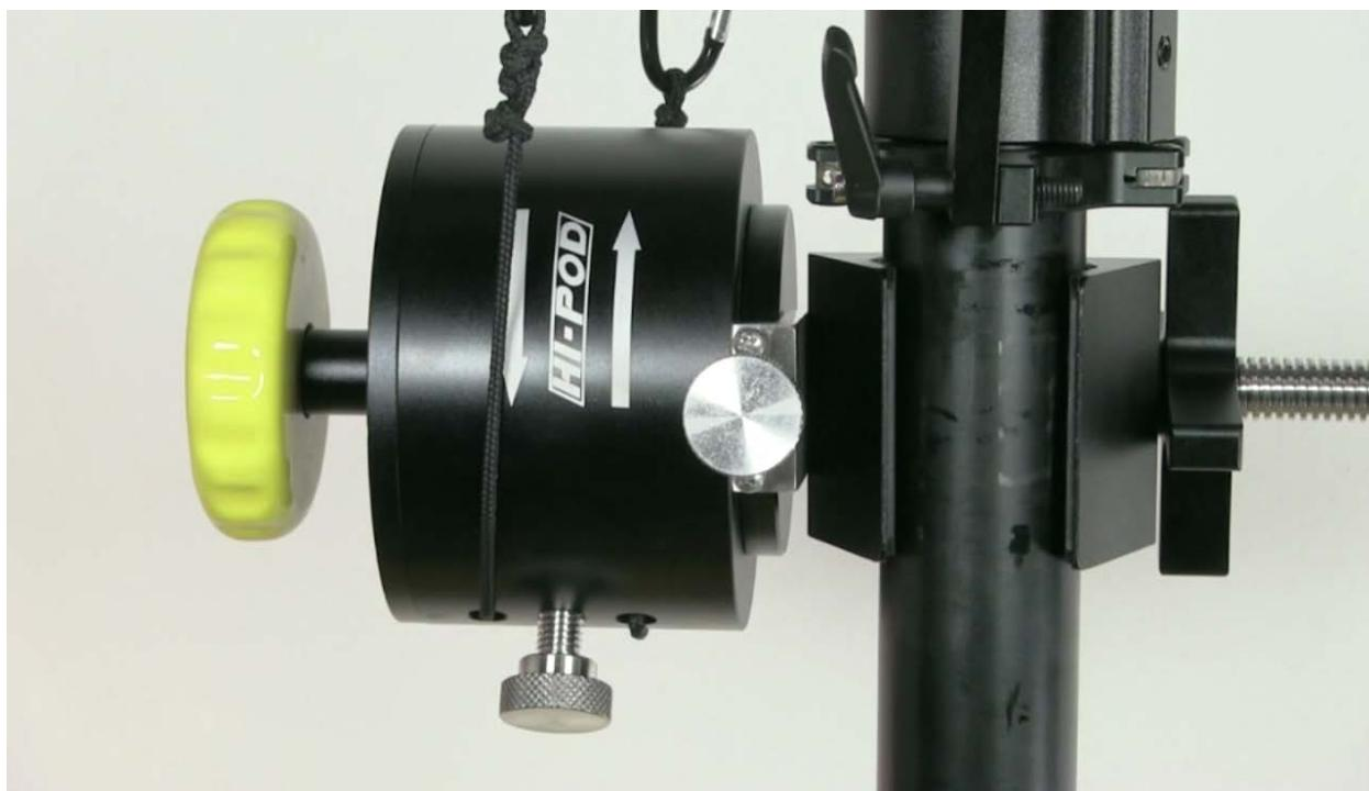
Connect the ropes coming out of the handle to the matching shorter cords coming down from the Hi-Pod Head. This engages the system. Connect with the attached carabiners.
