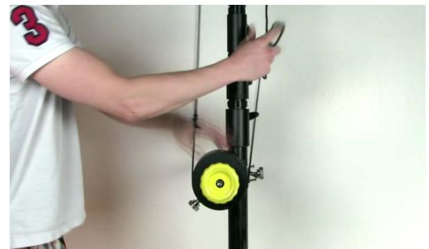
Notice, the rope connection for both the ADVANCED and PRO handles are the same. The two black ropes coming out of the bottom of the Hi-Pod handle, with a silver pin between them.
