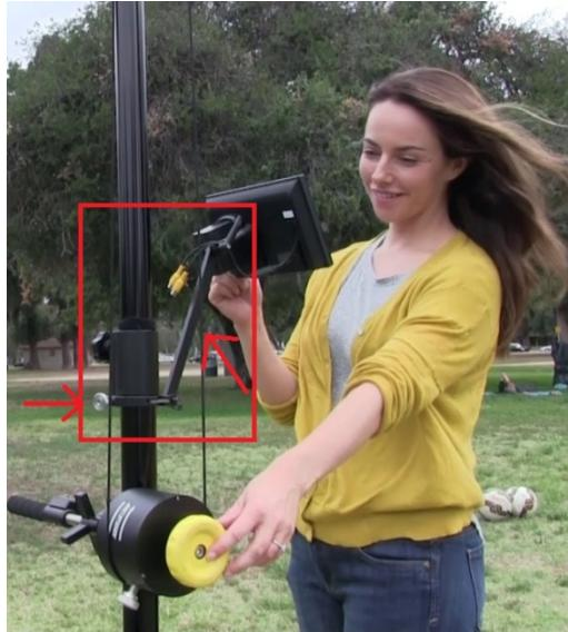
The LCD Mounting Bracket holds the screen on the tubes.
