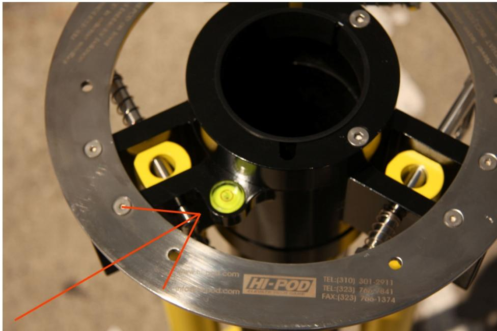
Always check the leveling bubble when setting up the HI-POD. The bubble must be level and the legs must be locked and solid.
