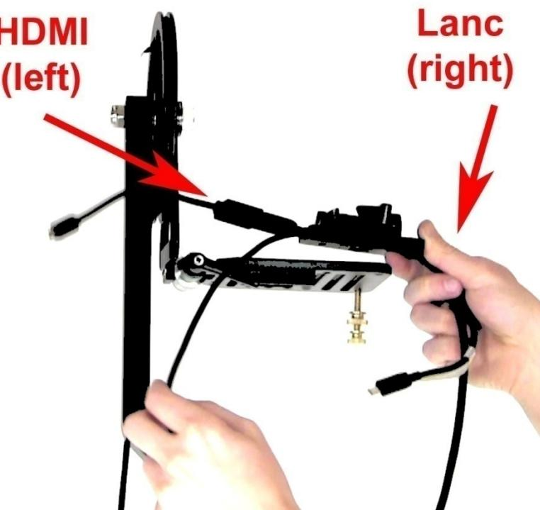
The HDMI cable will need to come out on the **left** side of the plate/head structure.
