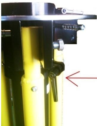
**IMPORTANT:** If you decide to split the base into three parts, when you put it back together you must make sure that the middle cylinder is locked to both the base plate (right), and to the leg bracket (left) – each secured by a twist lock.
