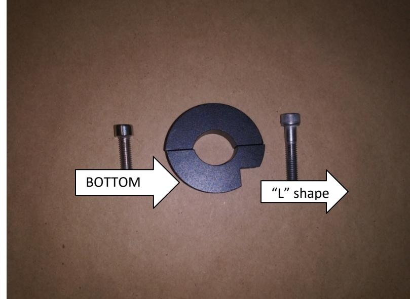
Tighten to the point where there is some mobility in the arm. Screw in bottom screw, and adjust placement of arm.
