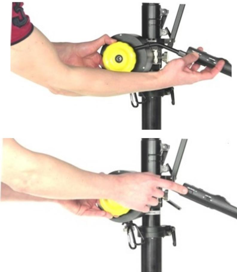
If you ever want/need to change the physical position of the remote, as it attached to the handle, you'll need to find an allen key (metric), open the screws, adjust the angle to your preference, and tighten again.
