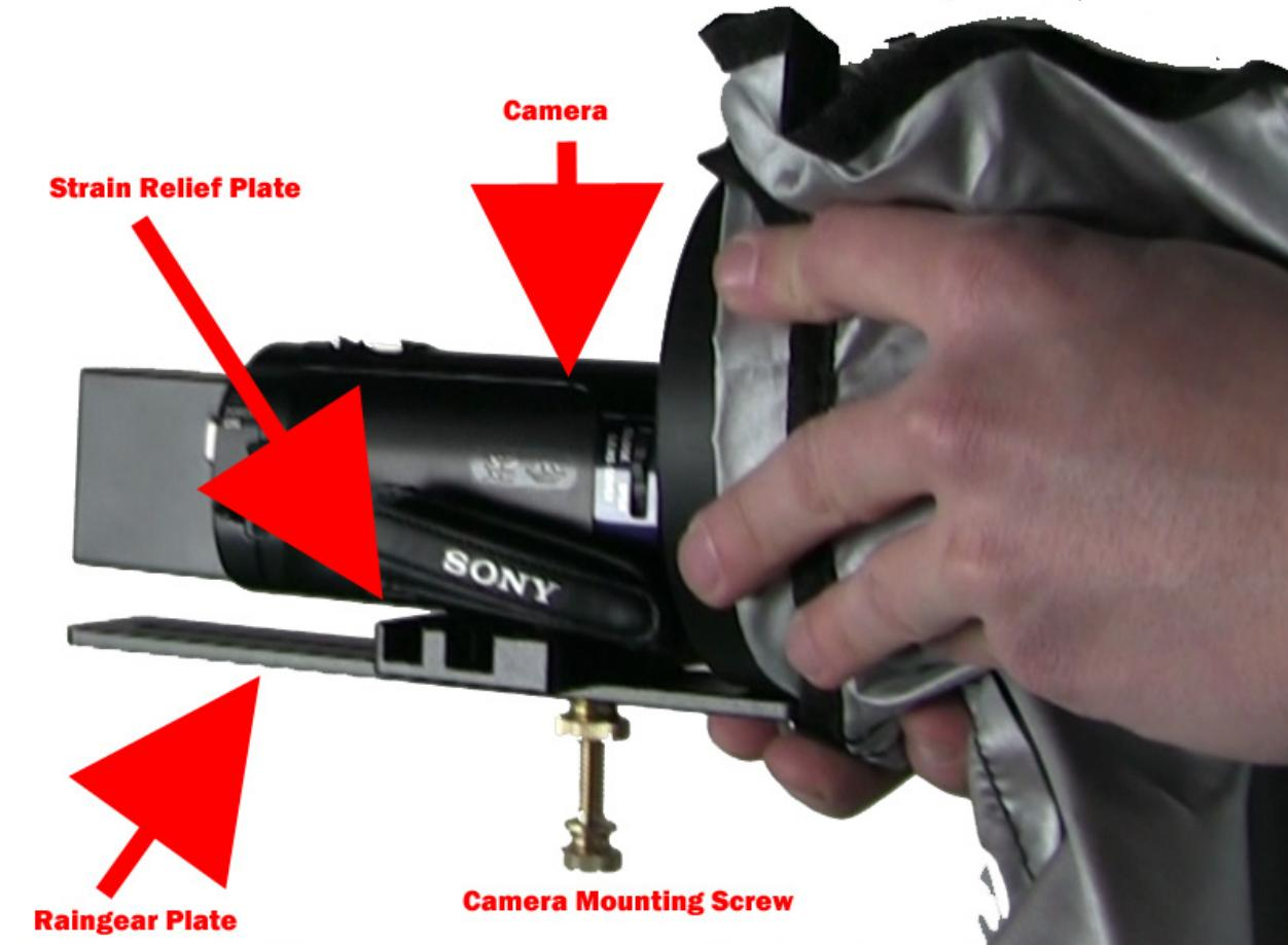
This image is shown without the wheeled head. The brass screw will be the only part under the wheeled head - everything else will go on top.
