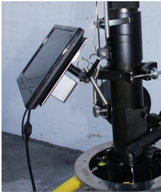
HI-POD PRO now includes a 10" HD LCD. We have created a new bracket to accommodate this new 10" LCD, as well as many different monitors. Not only is the bracket able to easily pivot up and down, but it's versatile enough to be moved up to another stage of tube. This allows very tall users to have more LCD placement flexibility.
