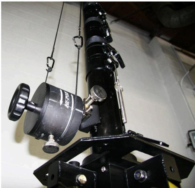
(2) Now that the handle is secure, notice the left hand side. It is a cylinder with a gripping wheel for your hand to grab & control the unit. Two ropes should exit the cylinder at the bottom, from either side of a large screw.
