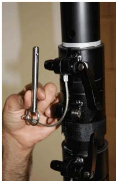
We have added an additional safety mechanism. Each locking collar for the tubes has the ability to receive a locking safety pin.
