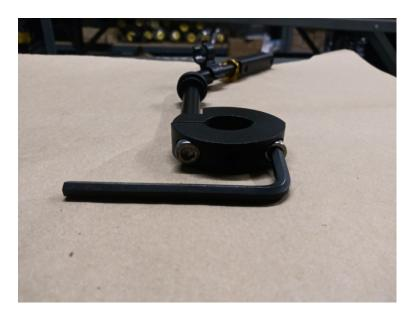
Once removed, place the split lock on the tubing between the yellow handle and the spool.
