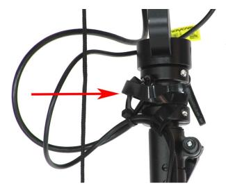
Then take the extra velcro and attach it around the tubes several times to keep it out of the way. This finishes mounting the cables, remote, and camera to the physical structure - with strain reliefs at each point.
