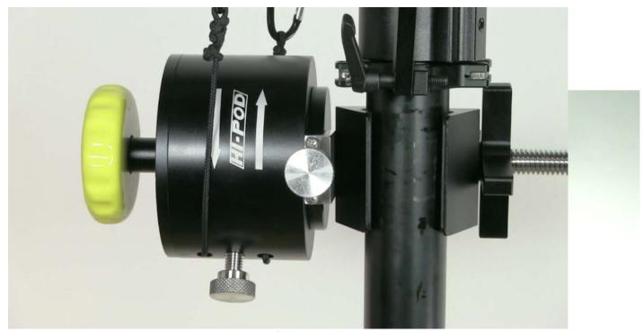
Connect the ropes coming out of the handle to the matching shorter cords coming down from the Hi-Pod Head. This engages the system. Connect with the attached carabineers.
