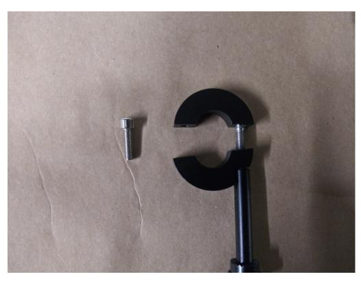
Tighten to the point where there is some mobility in the arm. Screw in bottom screw, and adjust placement of arm. Once comfortable position is found, tighten both screws to lock in place.
