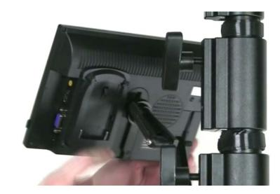
Once attached, tighten the round screw on the mounting tip behind the LCD to hold the screen in place.
