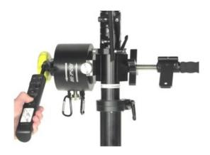
To mount the strain relief plate with quick release attached, use the smaller of the two middle holes on the bottom of the strain relief portion of the plate.
