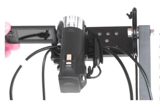
This image shows the camera snapped into the quick release plate. Pull back on the two levers on the quick release plate when it's time to pack up.
