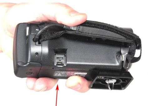
On the opposite side of the camera - under the hand strap - you'll find a small door. Open it and you'll reveal the 'Multi' port. This is where the cable will connect which sends signals to the camera from the remote control.
