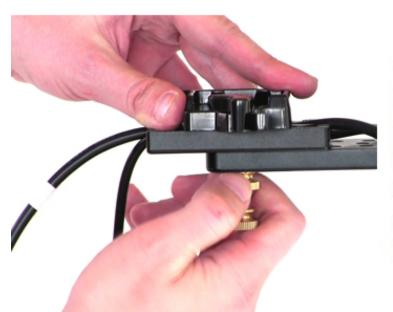
Then there is a secondary screw (see left) which comes up after the main screw is inserted which tightens this mechanism in place. Be aware that there are two parts of these screws, and both must be in place to hold tightly.
