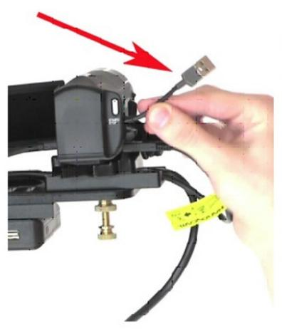
Now locate the small USB cable that is inside of the hand-strap for the camera. This is where you will connect the adapter cable.
