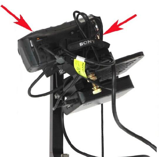
Then bind of the excess cable length of the USB adapter, and bind it inside of the camera handstrap. This keep the cable clean and out of the way so it won't catch on anything during operation.
