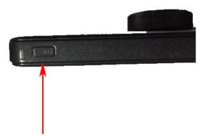
Click the button on the side of the battery to turn it on.
