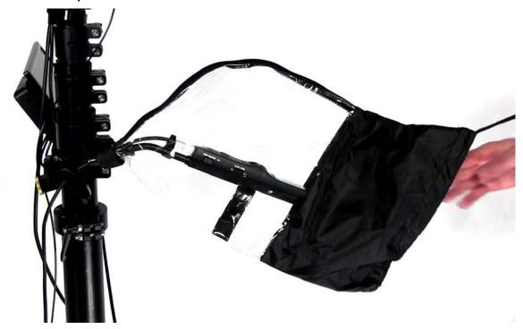
With the camera, lcd, and remote covered, this completes the raingear setup. If conditions vary, you can always go beyond what is included to enhance your protection.
