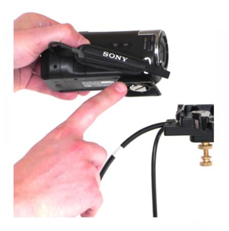
Notice how the camera already has a connection adapter attached to it. This is what you'll use to snap the camera to the quick release plate.
