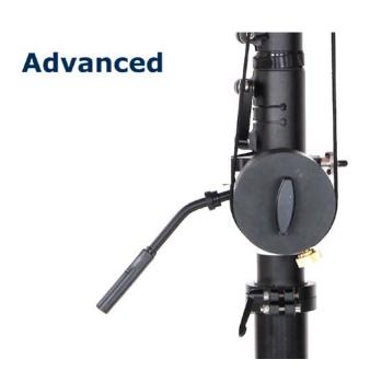
Note - each rope MUST go in opposite directions around the bottom of the handle. If this is not done correctly the handle will not be about to create the round motion which turns the head on top.
