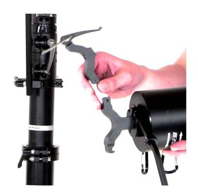
Open the clamp on the handle mount (image above), attach the handle to the core tubes, and close the clamp to hold it in place.
