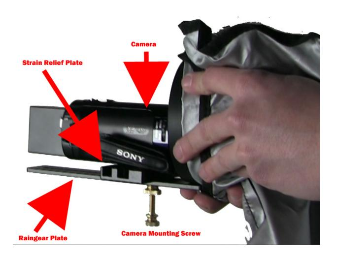
This image is shown without the wheeled head. The brass screw will be the only part under the wheeled head - everything else will go on top. Use the same hole on the strain relief plate to attach the brass screw as you do with the raingear. Just make sure that now, the raingear plate is below the strain relief plate, but on top of the wheeled plate.
