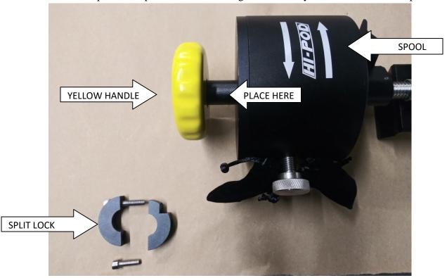
Have the "L" shaped notch facing towards you. Place longer hex screw through the access point. When placing split lock, start with the longer top screw. Screw in the remote by hand, this will allow you have more control for screwing the arm to the split lock.
