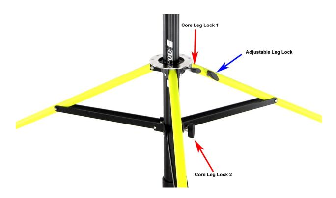
Once the black slats are level, turn the two knobs (shown in the above picture with red arrows) to lock the legs in place.
