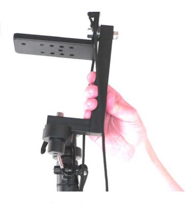
As mentioned the 'ADVANCED' head for the Hi-Pod mounts with the wheel on the <u>right</u> side of the tubes. The Handle mechanism will mount on the <u>right</u> side to match it.
