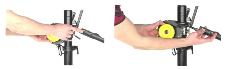
If you ever want/need to change the physical position of the remote, as it attached to the handle, you'll need to find an allen key (metric), open the screws, adjust the angle to your preference, and tighten again.
