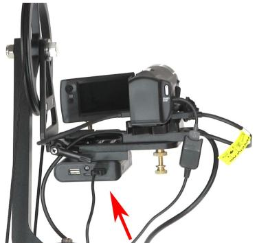
Then take the male end of the USB adapter and plug it into the USB power pack battery.
