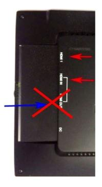
Take your standard sized HDMI cable and connect it to the top port (HDMI1) for video signal. Make sure the LCD is on the correct channel (HDMI 1, HDMI 2, etc) to display the video signal.
