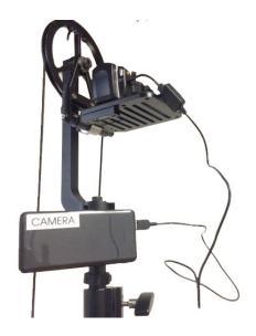
First, mount the battery to the tower (either to the top of the poles as shown or to the camera plate). Connect the battery to the camera with the female-to-male USB cable extension. The female end will connect to the USB cable found in the camera hand strap.
