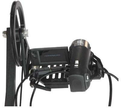
This image shows the camera snapped into the quick release plate. Pull back on the two levers on the quick release plate when it's time to pack up.
