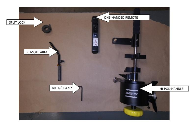
Using the Allen/Hex Key, loosen both internal hex screws. This will allow you to separate the split lock form the remote arm.
