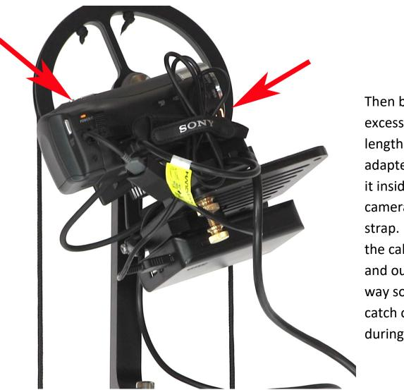
Then bind of the excess cable length of the USB adapter, and bind it inside of the camera handstrap. This keep the cable clean and out of the way so it won't catch on anything during operation.
