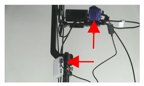
Find the USB power pack (exact style may vary but setup will remain the same), and attach to the tower where there is a hook at the top of the tubes. Use the brass screw (shown in the image) to sandwich the battery to the tower.
