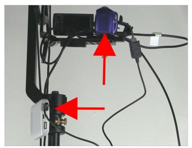
Connect the battery pack to the camera with a USB extension cable (included in your case). Note the shorter USB cable in the hand-strap of the camera, and use the longer extension to connect the camera/battery.
