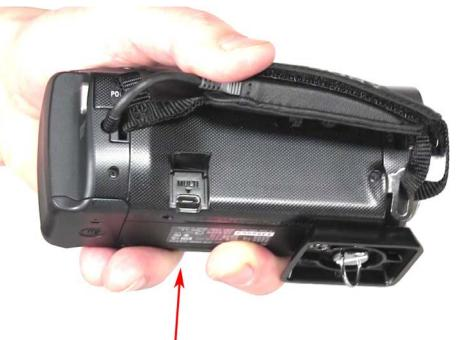
On the opposite side of the camera - under the hand strap - you'll find a small door. Open it and you'll reveal the 'Multi' port. This is where the cable will connect which sends signals to the camera from the remote control.
