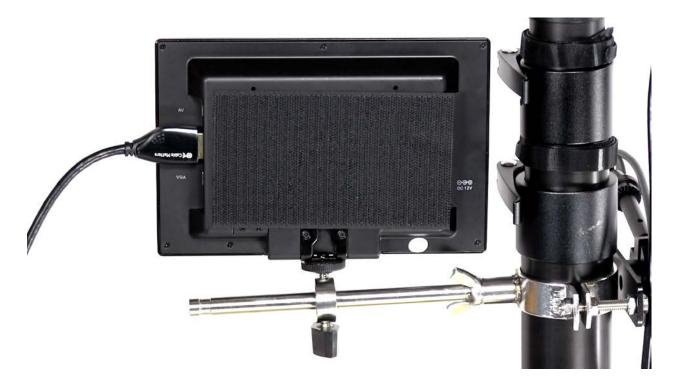
Find the larger LCD battery (with velcro pre-attached) and stick it onto the back of the screen.
