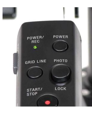
button light up on the remote - so the client believes everything is connected correctly - but then they have no control over zoom and record functions. This means you only have a half-connection of the cable into remote - enough to receive power, but not enough to communicate signals back and forth. Correct this by adjusting the placement of the white strain relief back onto the cable head, and make sure it is fully connected. Then everything will start working.
