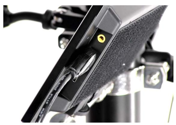
Connect the standard sized HDMI cable at the bottom of the cable bundle to the port.
