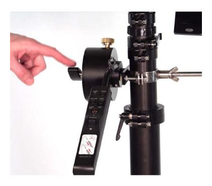
You'll also find a brass screw on top. If tightened this screw prevents the rope that's attached to a carabineer from pulling out of the black cylinder. If unlocked you can pull the rope out. This rope is what you'll use to connect the handle to the head at the top of the tower.
