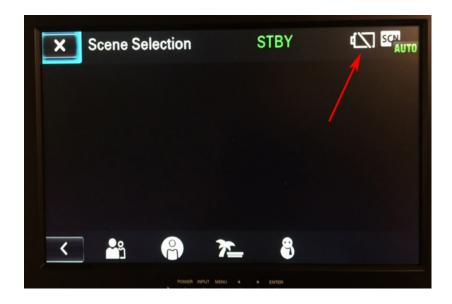
If your external battery is already connected (per instructions above) you need to 'click' the battery on to activate the power transfer. Sometimes the batteries don't automatically turn on (often they do -but not always). When the big USB battery takes over, the battery icon on the camera LCD will disappear. **This is what you want**.
