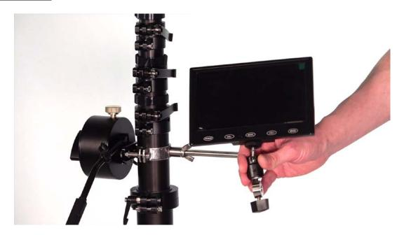
You'll find the LCD in the electronics bag. Note the metal part mounted beneath with an open hole (red arrow).
