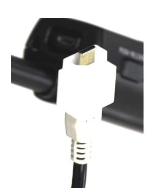
IMPORTANT: The white strain relief is NOT permanently attached to the cable head. It can shift backwards or forwards when the system is put away or when it sits in the case. If the white strain relief shifts forward on the cable head, the cable itself will not make a physical connection to the remote, and therefore will not function properly.
