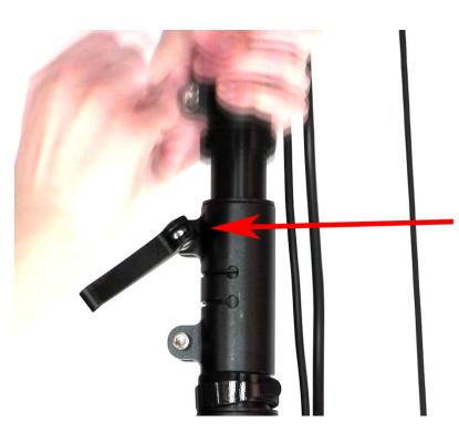
Note the lever (camlock) which you'll use to release and lock the tube collars. Repeat this for all stages.
