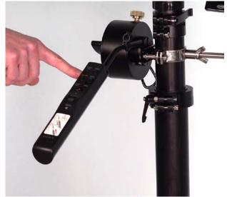
When ready to remove the remote, press the button on the left / top of the remote, and it will slide off.
