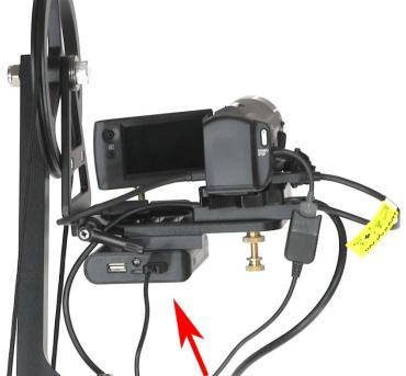
Then take the male end of the USB adapter and plug it into the USB power pack battery.
