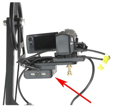
For this method you will take one of the brass screws as you did with the strain relief plate, and mount the camera battery with the reverse approach: battery will hang down under the camera plate, and the brass screw will connect from the top.
