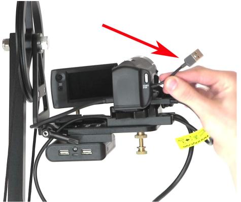
Now locate the small USB cable that is inside of the hand-strap for the camera. This is where you will connect the adapter cable.
