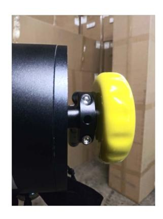
The rope locking screw must be pointing straight down.
