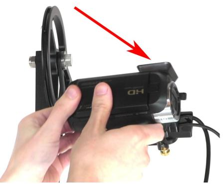
Notice how the camera already has a connection adapter attached to it. This is what you'll use to snap the camera to the quick release plate.
