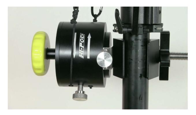
Connect the ropes coming out of the handle to the matching shorter cords coming down from the Hi-Pod Head. This engages the system. Connect with the attached carabineers.
