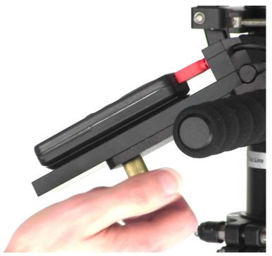
Once you have the top pin connected and the bottom hole lined up, take the brass screw and lock the remote into place.
