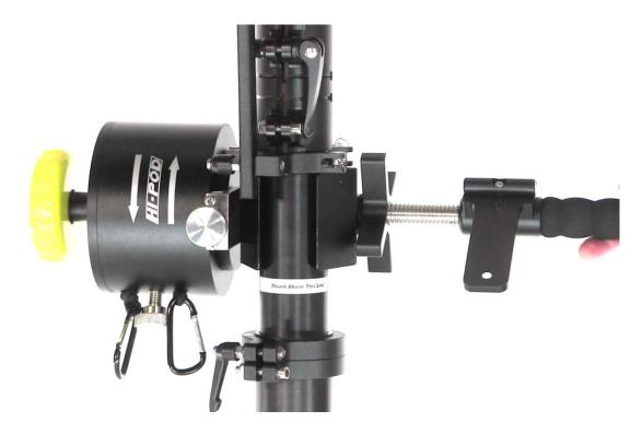
The reason you need to mount both the handle and LCD bracket above the white line can be seen in the image below. When you rotate the handle there needs to be enough clearance between the handle and the collar with ratchet (below the white line). Otherwise, if not setup with appropriate spacing the parts will bump into each other when you're filming.
