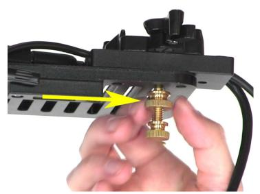
Then there is a secondary screw (see left) which comes up after the main screw is inserted which tightens this mechanism in place. Be aware that there are two parts of these screws, and both must be in place to hold tightly.
