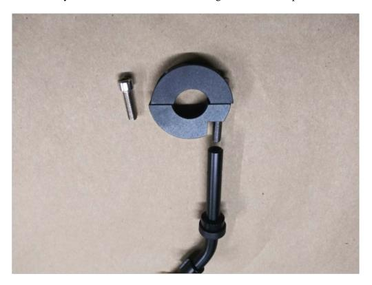
Following image should give you a better idea of how the split lock and screws must be placed.
