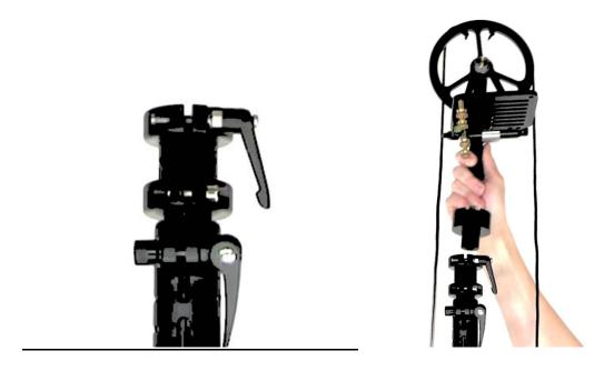
Once in place, use the ratchet at the top of the tubes to tighten and secure.
