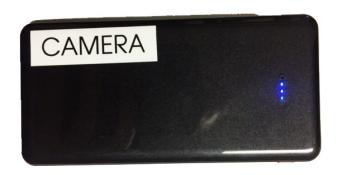
For those clients using either the grey or white USB batteries, you need to confirm that the battery is turned on and is set as the main power source before elevating. Without doing this, it's possible to leave the small internal camera battery active which will die quickly.
