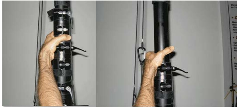
There are 5 collars for the 6 HI-POD tubes, each collar squeezing the upper tube. When you reach the recommended height you will see a white line. This white line tells you to stop elevating and lock the collar. It is not possible to push the innermost tube so high that it comes out. There is a built in safety catch that prevents the tube from coming out.
