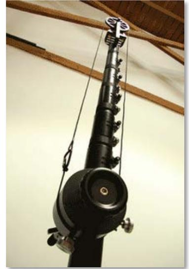
As you spin the X screw you are squeezing the clamps against the tube. Reverse this to loosen the handle later on.
