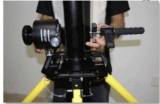
Connect the ropes via the carabineer clamp. The carabineer connectors make it very easy to attach and detach the handle from the tubes.
