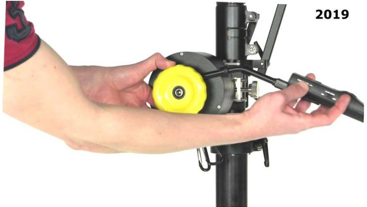
If you ever want/need to change the physical position of the remote, as it attached to the handle, you'll need to find an allen key (metric), open the screws, adjust the angle to your preference, and tighten again.
