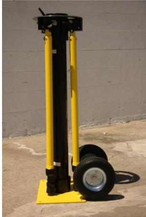
The base has 3 legs with redundant leg locks for added safety. Please examine the location of the pin. There are two holes that the safety pin can occupy. The first pin hole locks the leg closed. This is important when traveling, as it keeps the legs from falling out of place.
