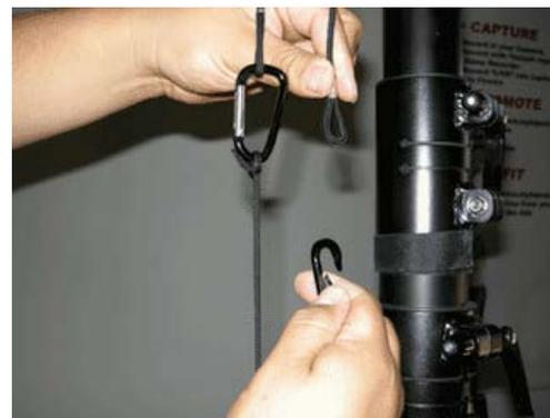
**Connecting:** As you face the HI-POD Handle, make sure the large silver screw & ropes are pointed towards the ground. Now, grab the rope that is closest to the tube. Pull that rope towards you. It will extend from the cylinder. Pull approximately 1 foot of rope, making sure that the large screw is still pointing down. With your other hand grab the other rope. Make sure this second rope is extending from the opposite side of the cylinder. Pull out the same amount of
