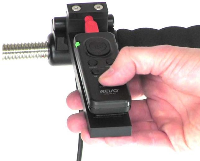
Once the remote is connected to the camera it has a light on it that will switch from red to green during operation. This is a really nice feature that removes the need to apply text/record data directly on the LCD. However, we will show those steps later in this method if you still want the info on the screen.
