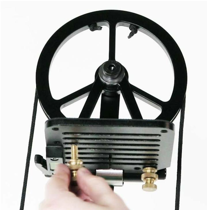
Take one of the brass camera mounting screws (attached to the plate of the head), and insert from below the plate with grooves carved out of it. You'll likely need to use one of the most exterior slots to mount.
