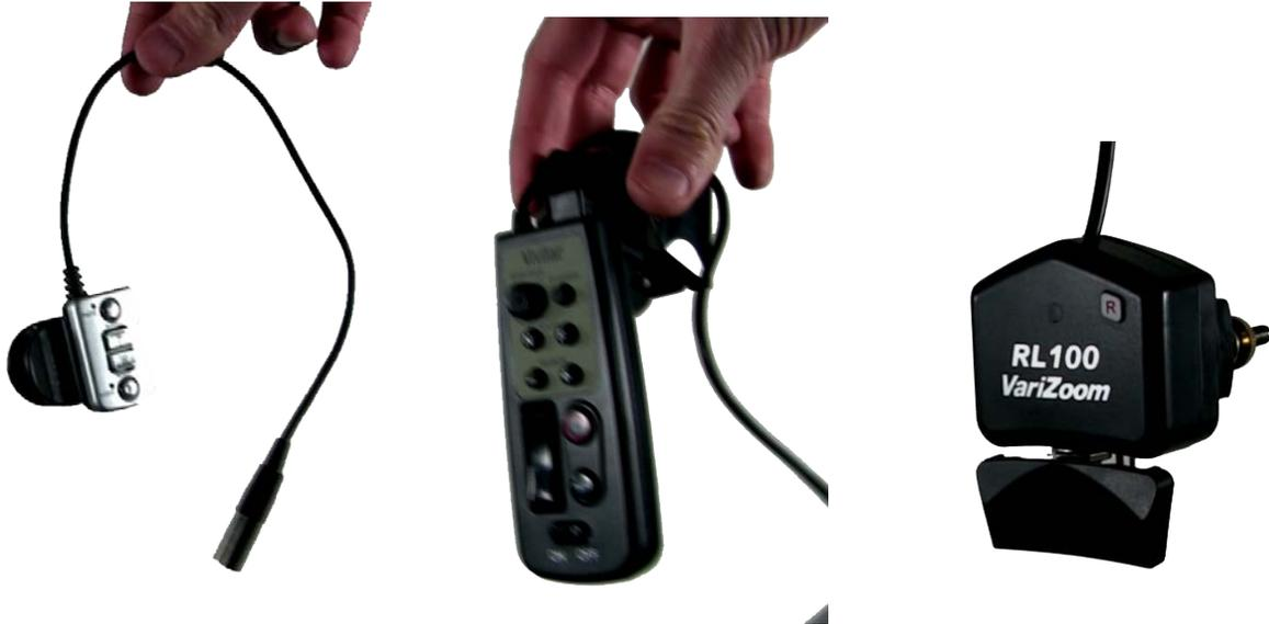
All of these remotes have a 4-6" cable which ends in a silver connector with three pins. This will connect to the long 'lanc' cable on the end which has ports to receive these three pins. Just connect the ends, and they will snap into place. You can release by pressing the small black button when disassembling.
