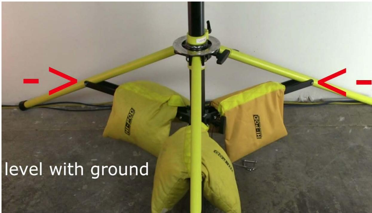
Once the black slats are level, hold them in position with the three yellow safety collars (see below). Once in place, these yellow collars will hold your leg position, while allowing the black knobs to stay unlocked, allowing the pole to turn.
