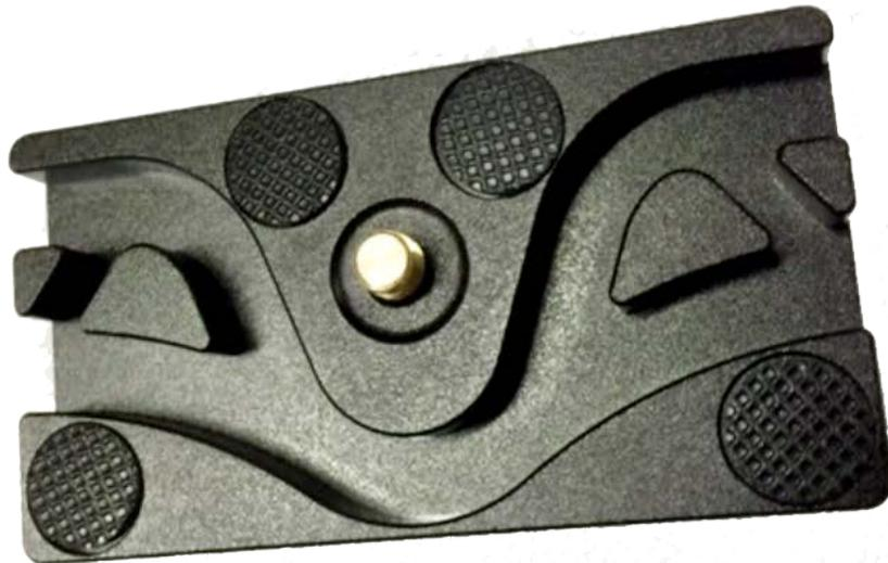
The Strain Relief Plate locks the video and linc cables firmly under the camera. When the unit is fully elevated, it prevents gravity from pulling down on the delicate cable tips/camera ports, which can cause the tips to break or ports to widen. If damage occurs your control/video signal will drop - so **USE THIS ITEM EVERY TIME.** *\*Damage to the system can occur as quickly as a single use if not applied.*
