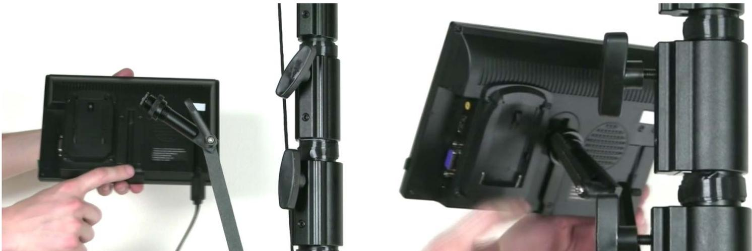
Once attached, tighten the round screw on the mounting tip behind the LCD to hold the screen in place.
