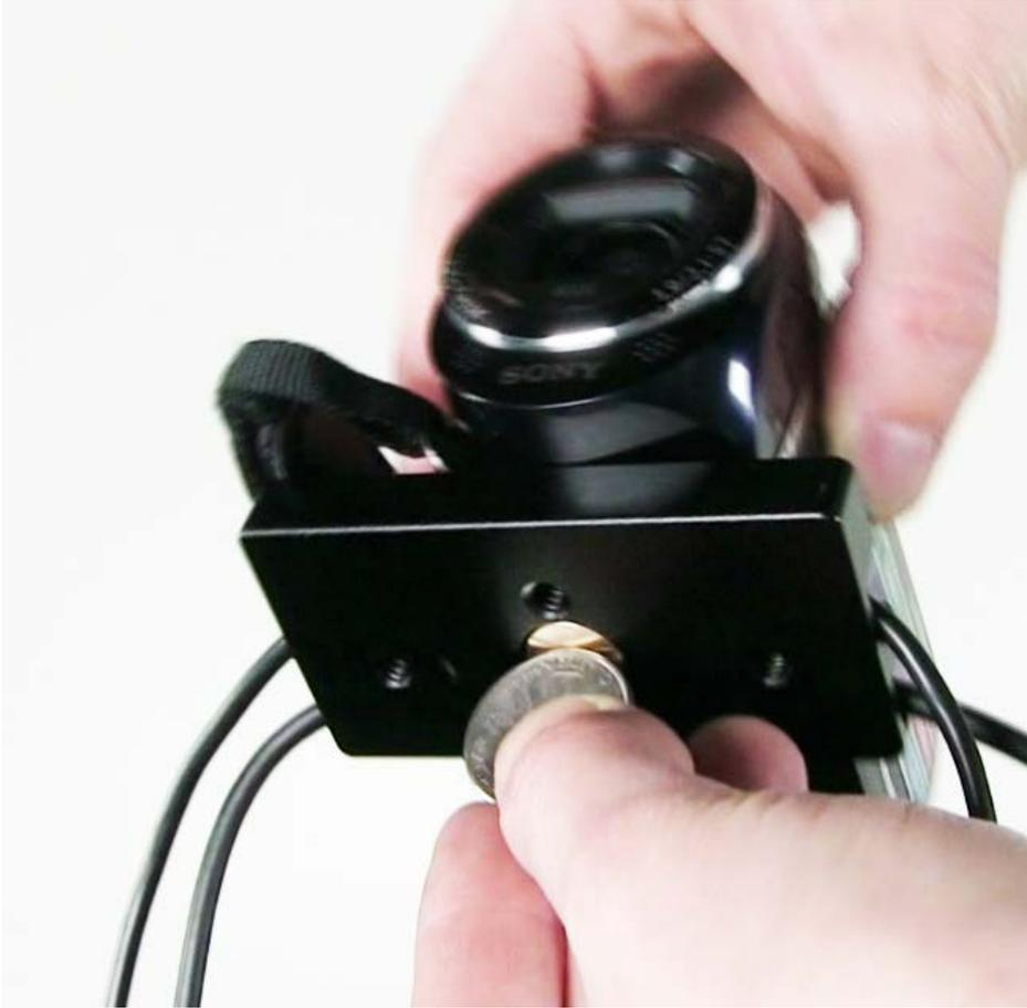
The brass screw is flushed against the bottom of the black plate, so you'll need to use a coin (or whatever is available) to securely connect.
