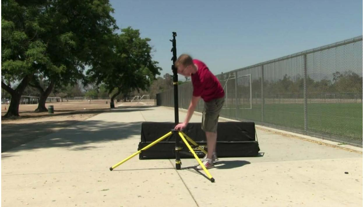
Take the tower out of your case, and place it on the ground. There are two black twist knobs on the base of the tower, and you will need to unlock these to allow for the tower legs to expand.
