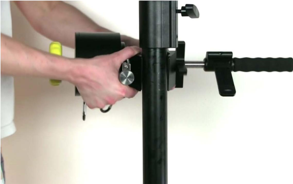
Find the Hi-Pod Handle in your case. Notice the two clamps that can open and tighten by turning the large black 'X' shaped piece on the item. Use this to attach the handle to the main pole.
